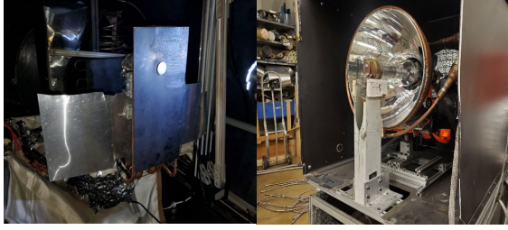
Fig.1: Gardon Gauge and Bulb/Reflector Assembly
